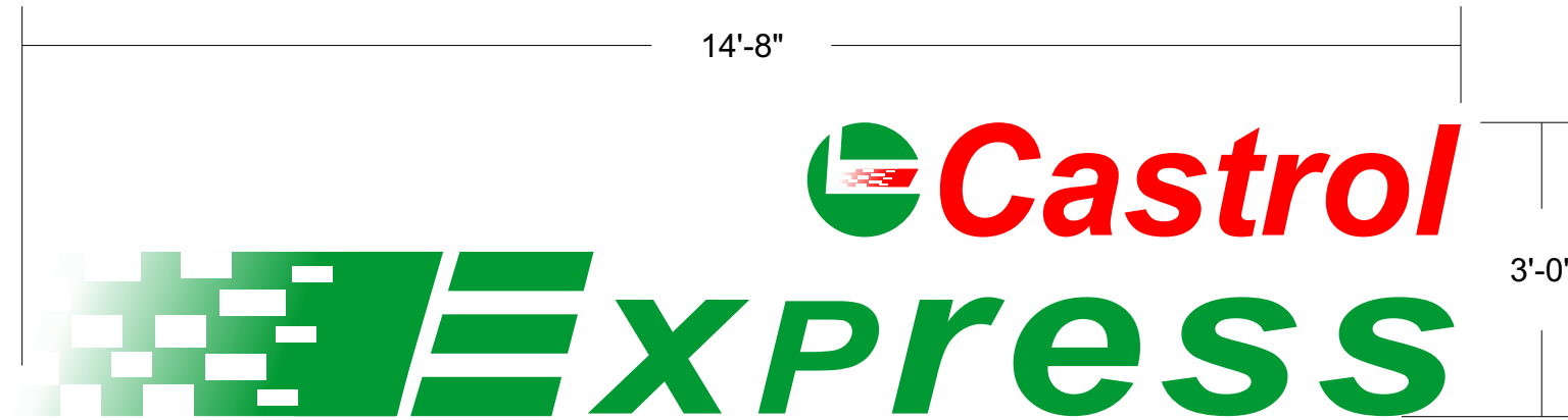
J CASTROL EXPRESS SIGN INTERNALLY ILLUMINATED FRONT VIEW SCALE: 1/2" = 1' 44 SQ FT QTY: TWO (2)
