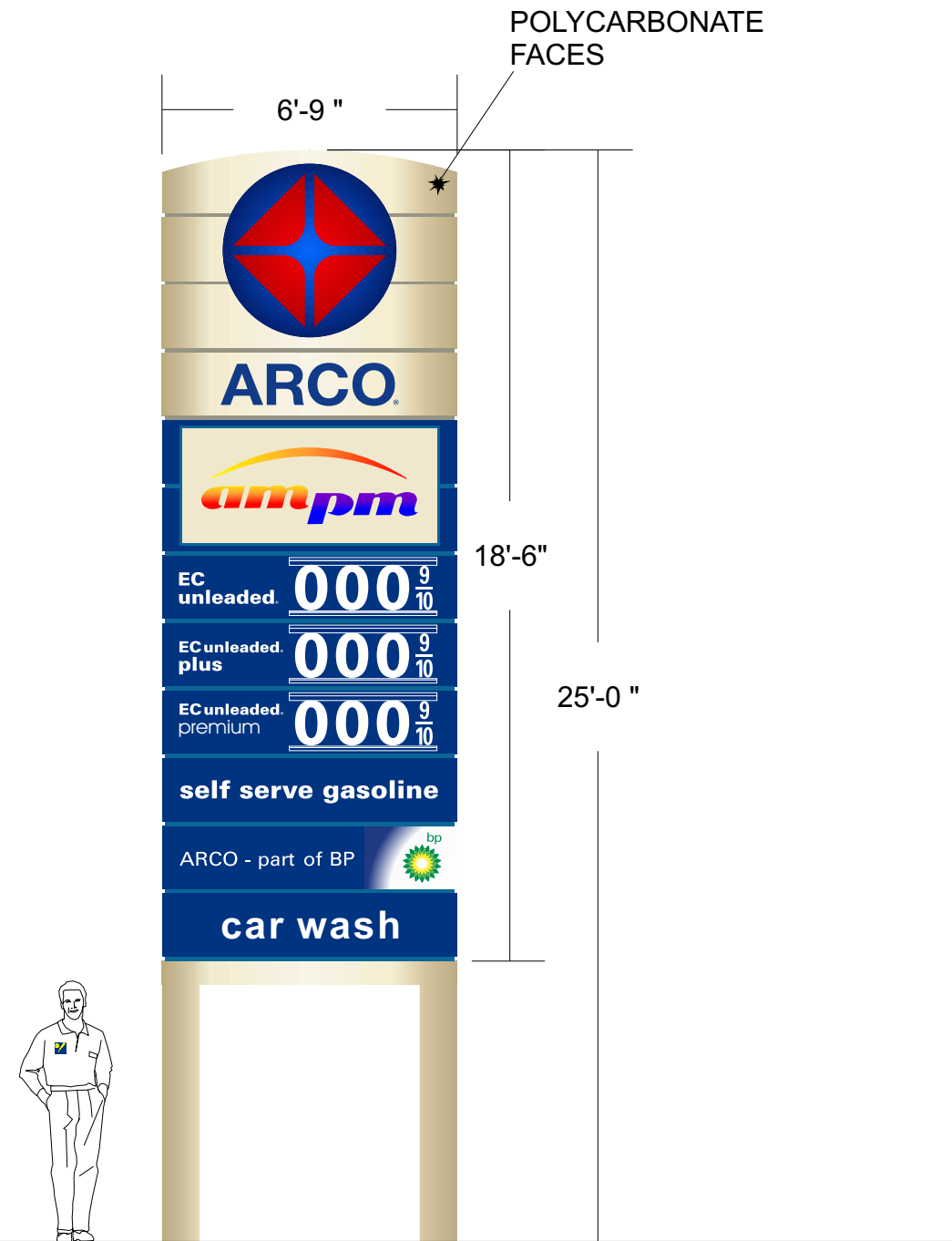
A ARCO NEW VISION TWIN POLE SIGN 125 SQ.FT. QTY: ONE (1) SCALE: 1/4" = 1' FRONT VIEW DOUBLE FACE INTERNALLY ILLUMINATED
