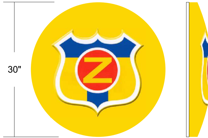
N 30" TRAVELZONE CANOPY SIGNS FRONT VIEW INTERNALLY-ILLUMINATED 5 SQ FT QTY: THREE (3)
